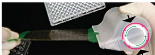
5. A brake mechanism in the dispenser hub prevents the film from extending farther than desired. To activate the brake, grasp more tightly with the hand holding the body of the dispenser.
