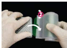
9. Seal the film securely on the microplate by pressing with the bottom of the round portion of the dispenser. The dispenser should now be ready for the next film application.
