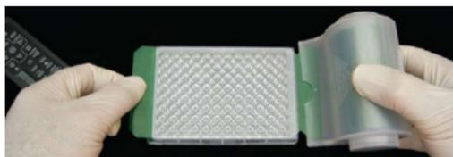
6. Holding the film lightly, so as not to stretch the film and introduce creases, lower the film and position it on the microplate.
