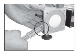
Use the face wrench with universal joint enclosed in the set of seals to assemble diaphragm clamping disc, diaphragm and diaphragm support disc (and eventually washers) to the connecting rod.
