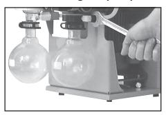
Use open-ended wrench to remove union nut on the fitting of the cover plate.
