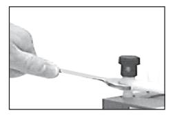
Use open ended wrench (w/f 15) to turn elbow fitting 1/4 of a turn, reconnect hose. Do not remove the elbow fitting from the pump head.
