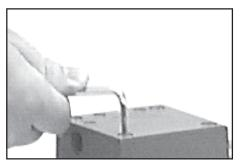
Use hex key to remove four socket head screws from pump head and remove upper housing (housing cover with housing cover insert and head cover).
