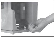
Use open-ended wrench to remove four cap nuts on the feet of the pump support and lift off pump together with pump support from the base plate.
