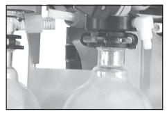
Remove union nut at the exhaust waste vapour condenser and remove hose from the inlet of the condenser.
