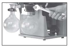
Use open-ended wrench to turn elbow fitting 1/4 of a turn, remove hose.
