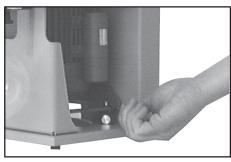
Position pump with pump support on the feet of the pump support and screw on four cap nuts.
