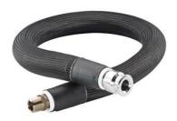
¾" ID Triple Insulated Flexible Hose has Welded-on S.S. Beaded Pipe Fitting for Connection to Reactor Inlet/Outlet. Uses CG-1968-69, 1 ½" BP Coupling (Sold Separately). Opposite End has ¾" Male NPT for Connection to Manifold Block.
