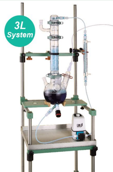
The compact 3 liter fits most laboratory hoods. It can also be used in walk-in hoods with the CG-1951-100 mobile or CG-1950-100 benchtop reactor stands.
