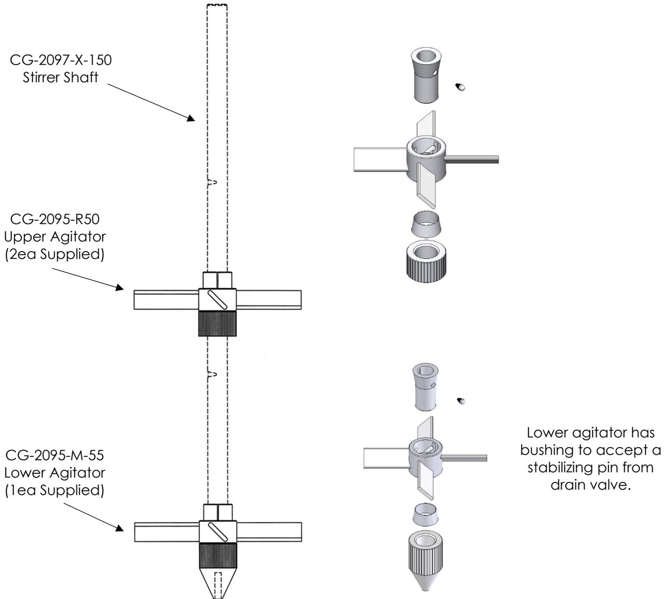
The stirrer shaft and agitators are assembled and installed when shipped. Use the following instructions should you need to remove or adjust these components.
