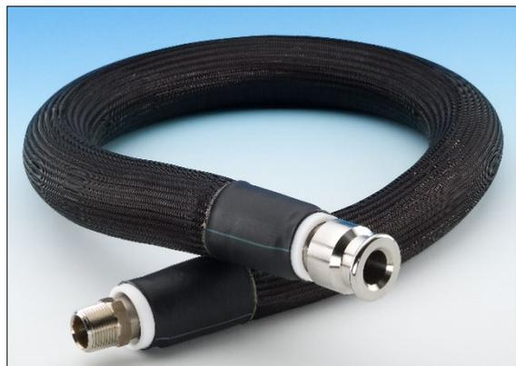
3/4" ID Triple Insulated Flexible Hose has welded-on S.S. beaded pipe fitting for direct connection to inlet/outlet. Opposite end is a 3/4" Male NPT for connection to manifold block.
