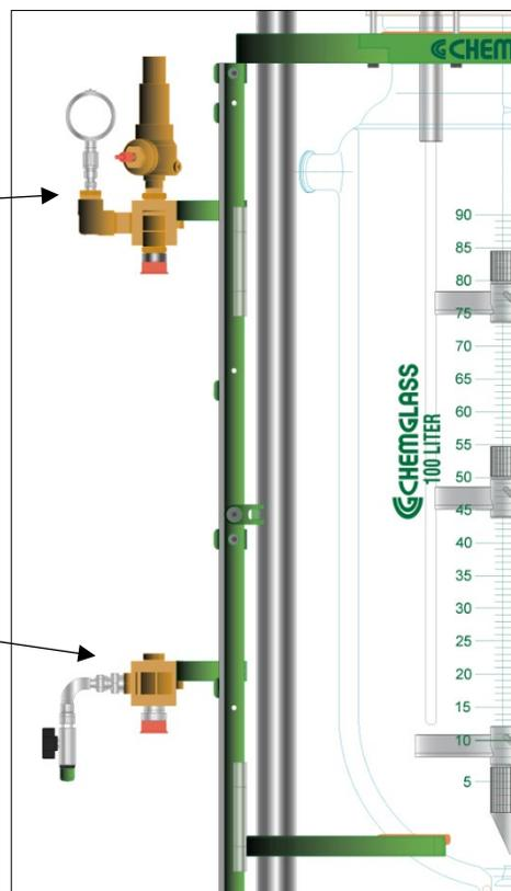
The high flow manifold system and triple insulated flexible hoses are assembled and attached to the inlet/outlet jacket connections when shipped. Use the following instructions should you need to remove or adjust these components.
