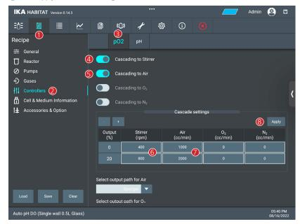
Option 2: To have DO control by stirrer speed as the first step, and then the gas flowrate adjustment in the second step.
