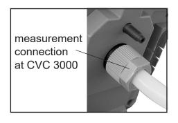
Condensate and deposits will affect the measurement results. Clean the pressure transducer, if necessary. See section "Cleaning the pressure transducer", pg. 87.
