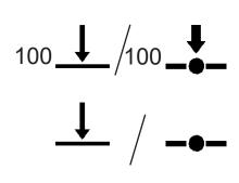
Vacuum control to a preset vacuum value (here: 100 mbar/Torr/hPa); (without / with VACUU•BUS-compatible VARIO pump)
