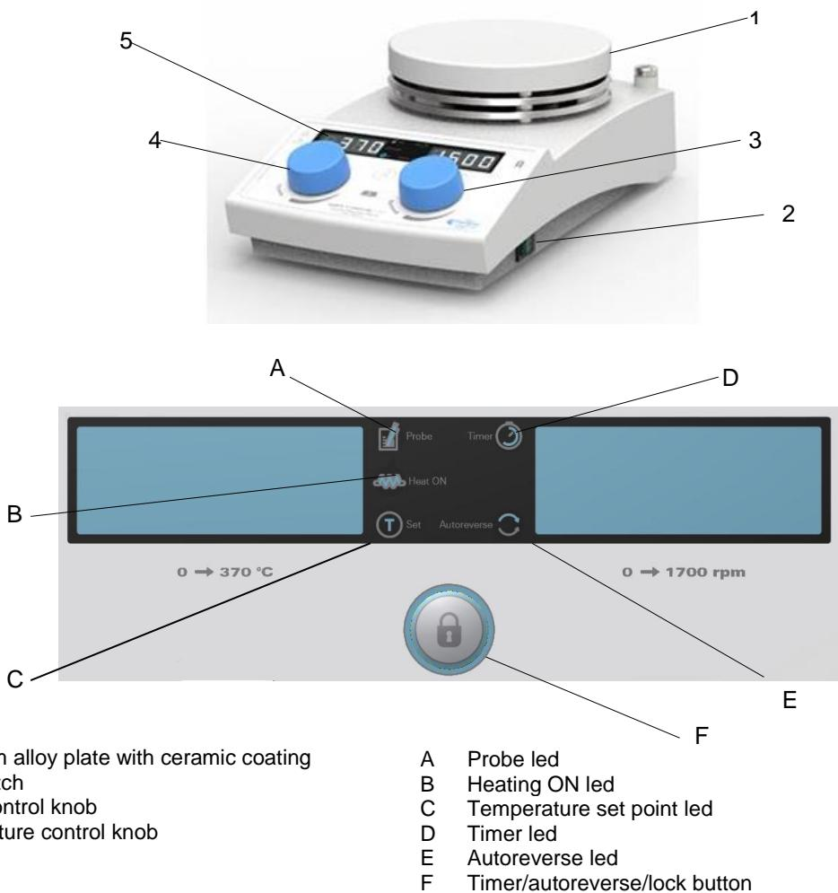
The Aluminum alloy heating plate with ceramic coating (1) ensures:
