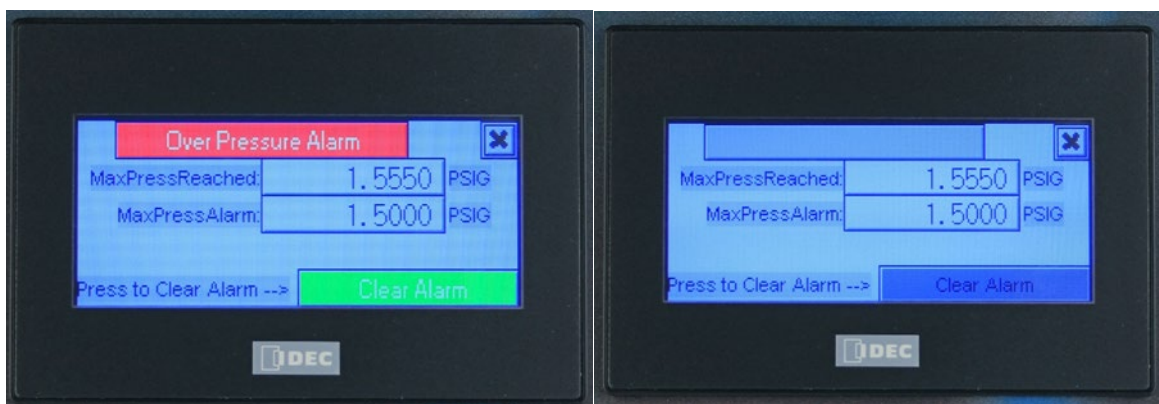
Figure 23 – Max Pressure Alarm
