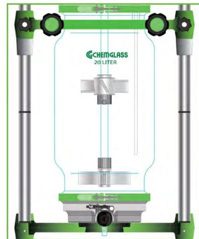
\*NOTE: THE BOTTOM IMPELLER SHOULD NOT BE RUBBING ON THE FILTER\*
