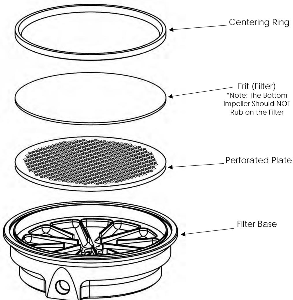
1. Place the o-ring in the beveled edge of the filter base.
