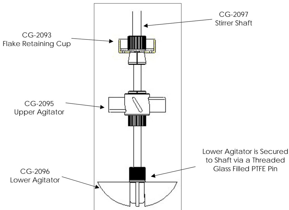
The stirrer shaft and agitators are assembled and installed when shipped. Use the following instructions should you need to remove or adjust these components.
