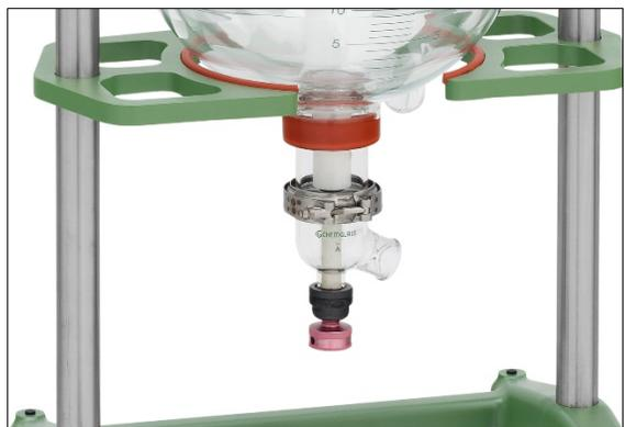
**WARNING: PLEASE NOTICE TEMPERATURE LIMITATIONS ON O-RINGS LISTED BELOW BEFORE USING THIS VALVE. PLEASE USE THE CORRECT O-RING FOR THE TIP BASE ON YOUR APPLICATION TEMPERATURE.**
