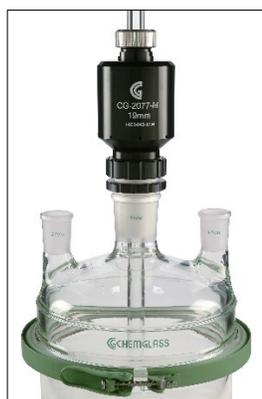
Mechanical Seal Stir Bearing
