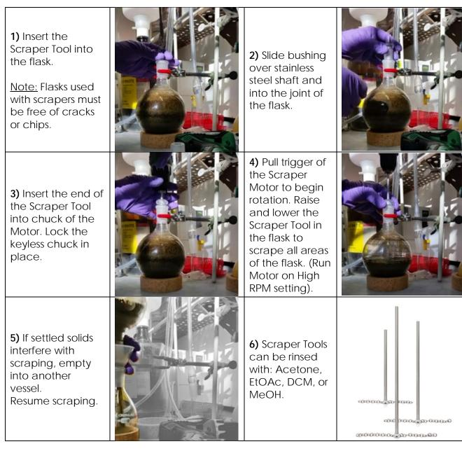
NOTE: Chem-spin tools must only be used with the correct corresponding flask size/capacity.
