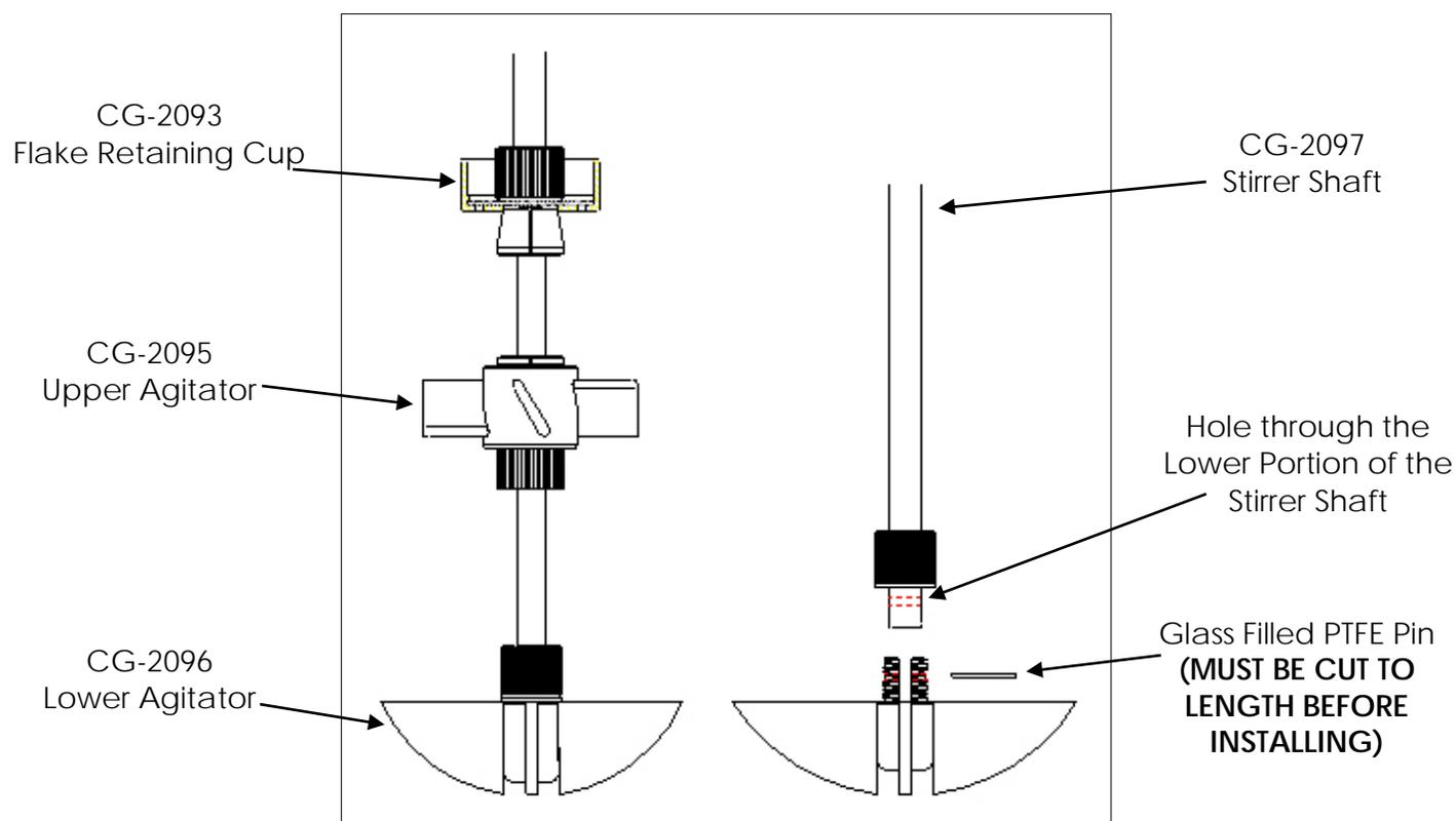
The stirrer shaft and agitators are assembled and installed when shipped. Use the following instructions should you need to remove or adjust these components.
