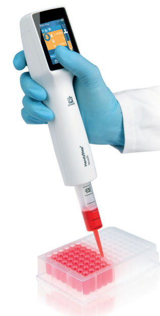
Multi dispensing with the HandyStep® touch and PD-Tip™ //
