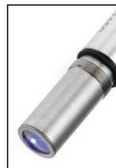
Blue light: A decisive part of the VISIFERM™ measurement principle.
