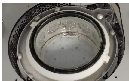
Double glass walls of the reaction chamber keep reaction vials at the correct temperature.
