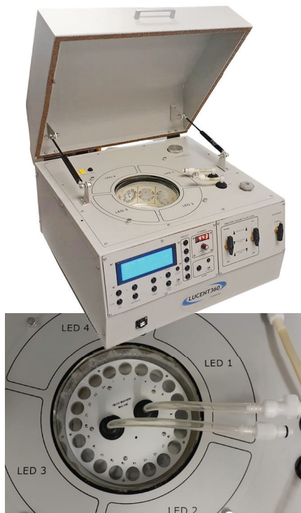
Reaction vials can be thermostatically controlled (0° to 80° C) via a standard heater / chiller unit.
