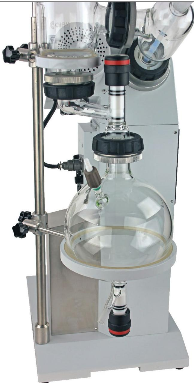
**5. Install 3L Receiving Flask (CG-1334-X54) and Flask Holder.**
