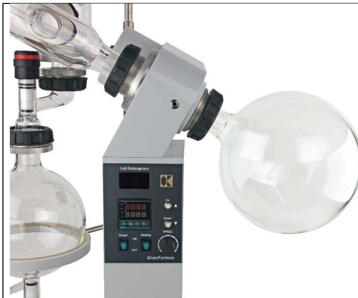
**6. Install 5L Evaporating Flask (CG-1334-X52).**
