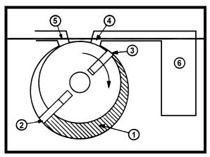
This expansion/compression cycle constitutes one complete cycle of the pump operation. This cycle is repeated as the vane (2) passes the intake port and seals it against the atmosphere. Therefore, two pump cycles are performed during each revolution of the pump rotor.
