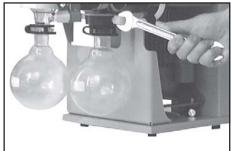
Use open-ended wrench to reconnect hose to elbow fitting.
