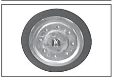
Check for washers under clamping disc. Do **not mix** the washers from the different heads. Make sure that the original number is reassembled at the individual pump head.
