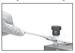
Use open ended wrench (w/f 15) to reconnect hose to elbow fitting.
