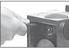
Use face wrench to remove diaphragm support disc.
