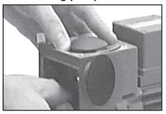
By turning eccentric bushing (front of connecting rod), bring connecting rod into a position in which diaphragm is in contact with housing and centred with respect to bore.
