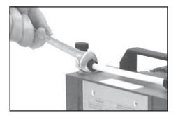
Tighten union nuts first by hand and then tighten one full turn using open ended wrench.
