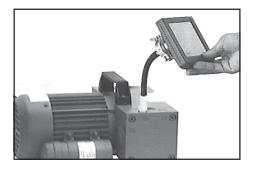
By measuring the pressure at the inlet port of the individual head: Use a suitable vacuum gauge (e. g. DVR 2, cat. no.: 68 29 02), make sure that it is correctly calibrated, and measure the pressure at the inlet port. A vacuum of less than 90 mbar should be indicated.
