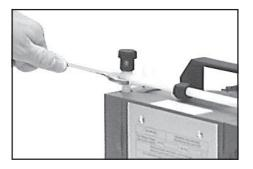
Use open ended wrench to turn elbow fitting 1/4 of a turn, reconnect hose. Do not remove the elbow fitting from the pump head.
