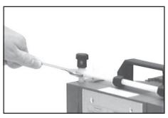
Use open ended wrench to reconnect hose to elbow fitting.
