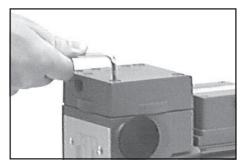
Use hex key to remove four socket head screws from pump head and remove upper housing (housing cover with housing cover insert and head cover).
