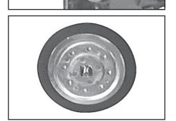
Check for washers under clamping disc. Do not mix the washers from the different heads. Make sure that the original number is reassembled at the individual pump head.
