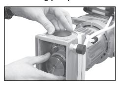
By turning eccentric bushing (front of connecting rod), bring connecting rod into a position in which diaphragm is in contact with housing and centred with respect to bore.
