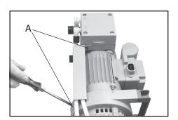
➡ Remove cover plate. Use Phillips screw driver size 2 to loosen screws (A). Pay attention to lock washers.
