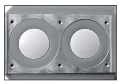
Bring diaphragm into a position in which diaphragm is in contact with housing and centred with respect to bore.
