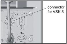
The cable of the gauge head is connected to the female connector at the rear side of the vacuum controller.
