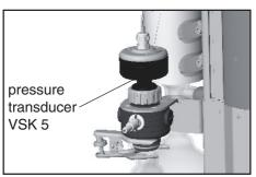
Max. permitted pressure at the pressure transducer: 2 bar (absolute).
