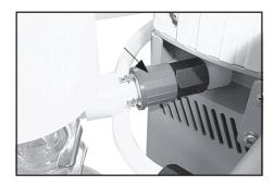
Remove union nut at the condenser and remove hose from the inlet of the condenser.
