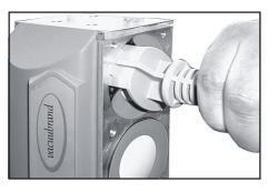
Make sure that the square head screw of the diaphragm clamping disc is correctly seated in the guide hole of the diaphragm support disc.
