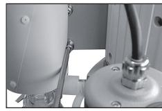
Unscrew the exhaust waste vapour condenser from the pumping unit.
