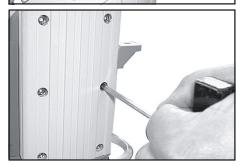
Use hex key to remove six socket head screws from pump head and remove upper housing (housing cover, housing cover insert and head cover).
