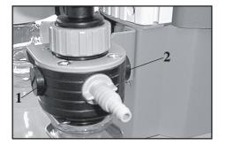
Hose nozzle (inlet of the pumping unit):
