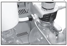
Use open-ended wrench to remove union nut at the inlet of the pump.
