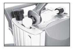
Use open ended wrench to reconnect hose to elbow fitting. Tighten union nuts first by hand and then tighten one full turn using open ended wrench.
