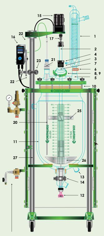
High Flow Manifold System Included M30 x 1.5 circulator fittings and insulated hoses, -60 to +200°C
