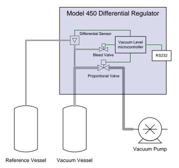
In the differential configuration, when the unit is in "REF" mode it will regulate the pressure in the vacuum vessel to the same pressure in the reference vessel
